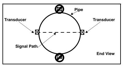
Figure 3-3: Desired Projection of Acoustical Signal Path
